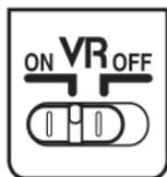
**Select ON to enable vibration reduction.** Vibration reduction is activated when the shutter-release button is pressed halfway, reducing the effects of camera shake for improved framing and focus.
